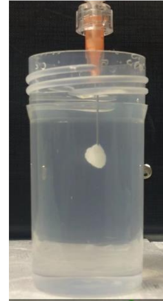
Silica-Silica composite depot after injection → reforms a gel
